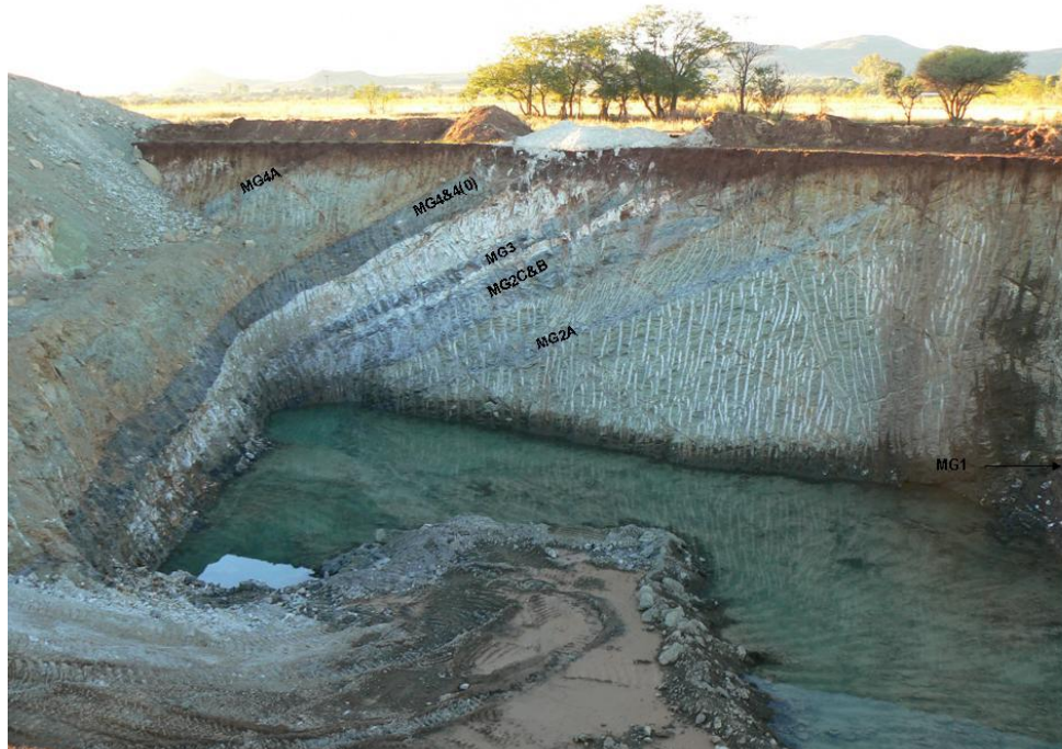
Figure 7.3_2 Photograph of Pit Sidewall showing the relationship of the various MG Chromitite Layers (Pit on Portion 286)
